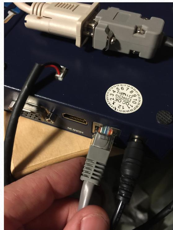
Connect the other end of the cable to the ethernet port on the computer.
