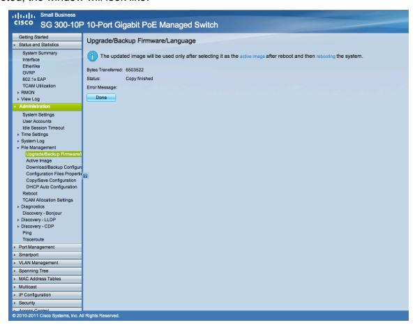
There are two firmware images on the Cisco SG-300. One is the "active" image that is presently in use on the switch. The second is a backup image. This is the image where your upload was just saved. We now need to switch to this new image as the boot image and then reboot the switch. In the File Management section of the left hand menu, go to "Active Image." The screen will look like:
