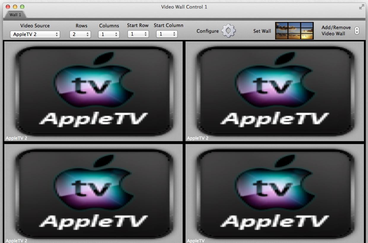
selected, enabling the video wall can be done in one of two ways. First the user can select the number of rows and columns as well as the start row and the start column of the combined image by using the pop-up menus in the tool bar. Once this is done, click the "Set Wall" button.
