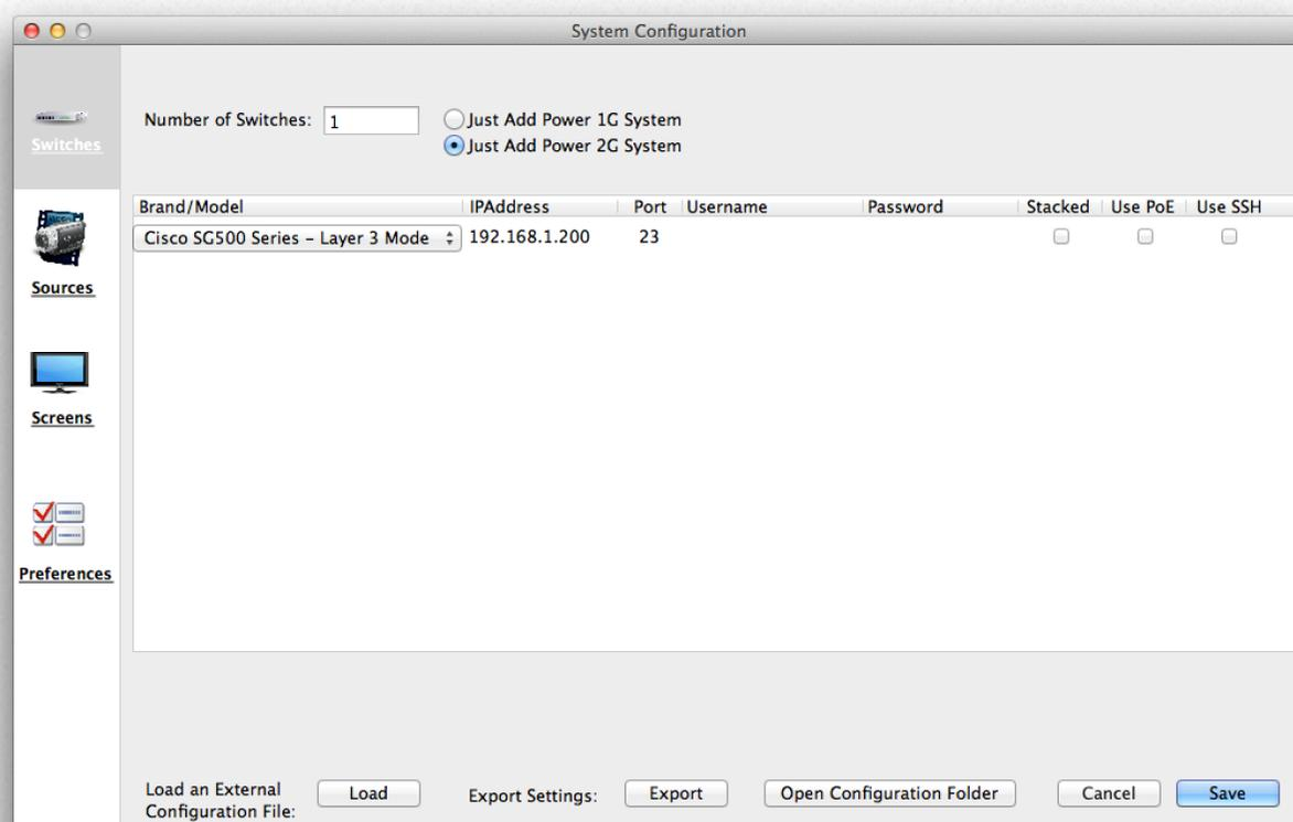
c.) Choose the brand of switch being used from the pull-down menu. Important: If a “Layer 3” architecture is being used, be sure to choose one of the “layer 3 mode” selections.
