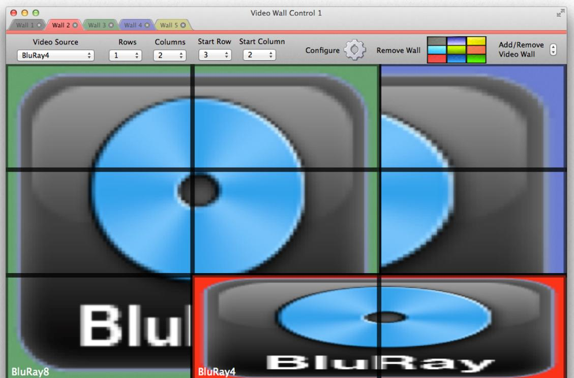
The video on the screens will adjust to show similar to what is being displayed in the software. Depending on the size of the video wall, it may take a few seconds for the changes to be made for all screens.
