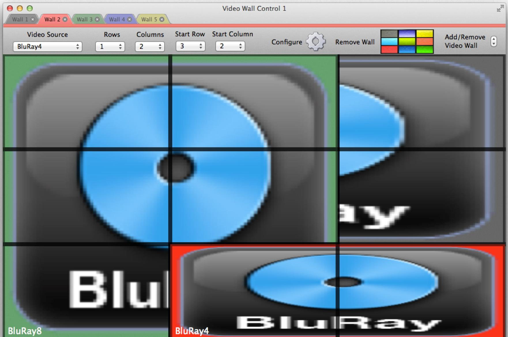
MediaSwitcher Wall Control is an add-on enabled by the license code entered for the software. The Wall control feature enables full dynamic video wall control of the Just Add Power hardware. MediaSwitcher's video wall control supports video screen matrix sizes of up to 16 rows and 16 columns. Multiple screen matrices are supported for systems that need control of more than one matrix of displays. For each set of displays, multiple video
