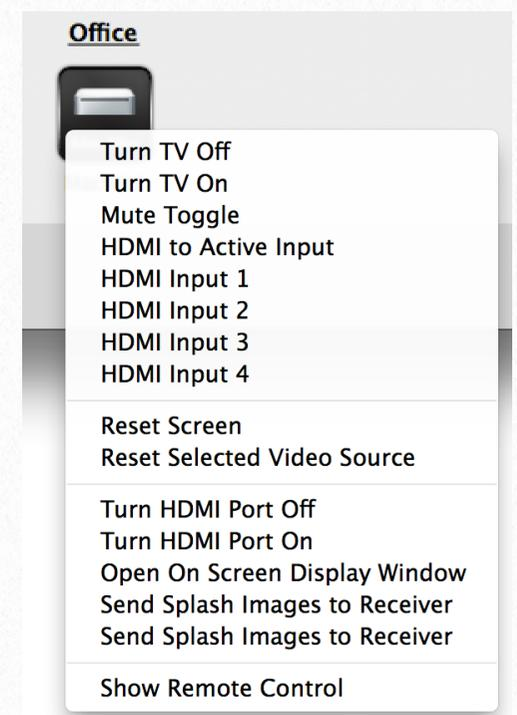
If the screen has a 2G+ receiver, additional options are given that will send CEC commands to the receiver to be sent to the TV. These commands are to set the HDMI input, turn the TV on and off and to toggle mute. Please note that not all TVs work with all CEC commands. It can be hit or miss. MediaSwitcher is not at fault if some commands do not work.
