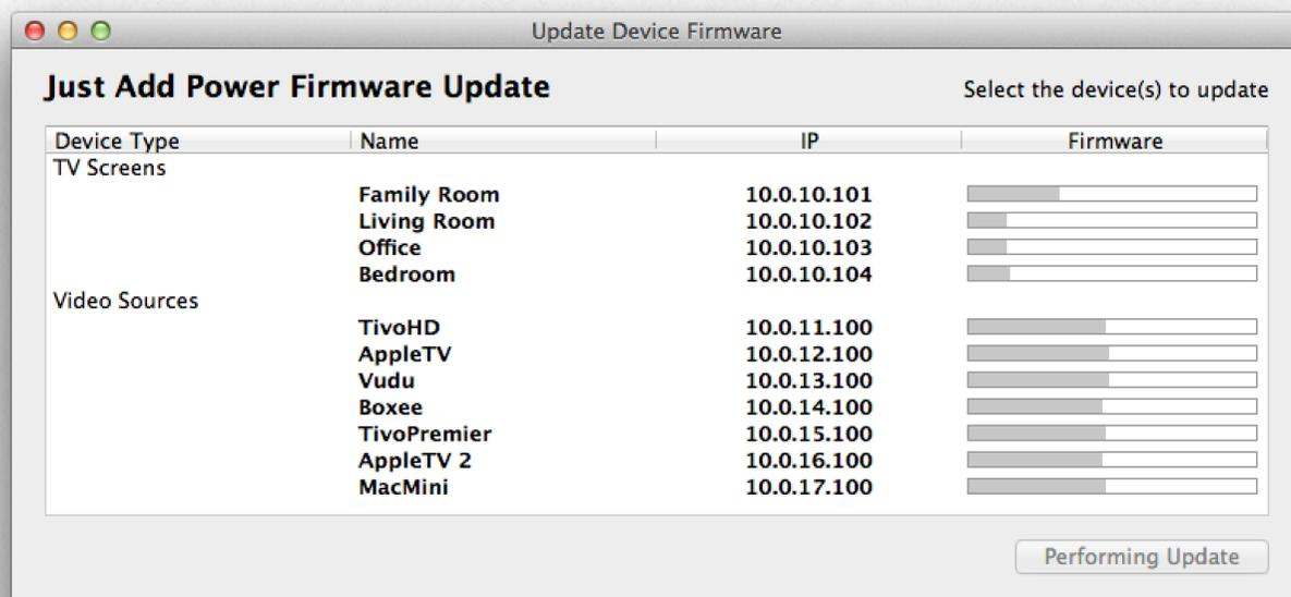
When a device has finished, it reboots. This is noted in the firmware column. Once the device has restarted, MediaSwitcher will connect to the device and show the new firmware version in the Firmware column.
