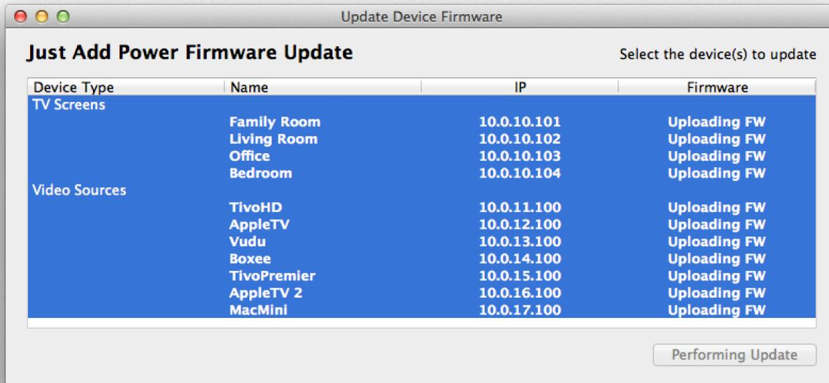
Once the firmware has been uploaded to the hardware, the update process begins. Progress bars will appear in the firmware column showing the progress of the update.
