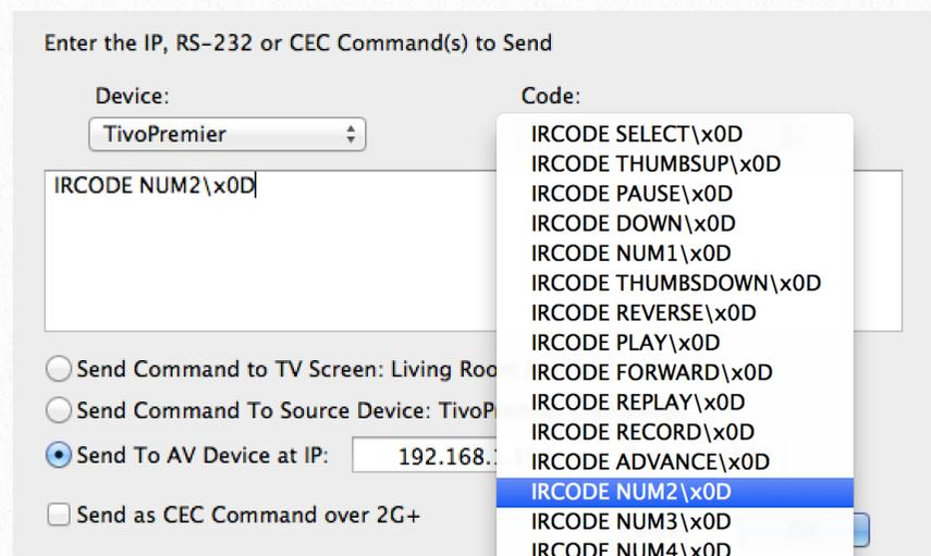
Once the code has been entered properly, click the “OK” button. The programming window will close. The button on the remote control panel is now updated. Click the next button to continue programming. Once programming is complete, press the escape key to exit learning mode.
