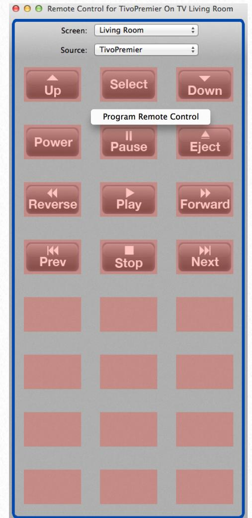
2.) Once in learning mode, the background of the remote control window will be shaded green and “Learning Mode” will be indicated on the window. Click on the desired button to be programmed. To exit learning mode, press the Escape key.
