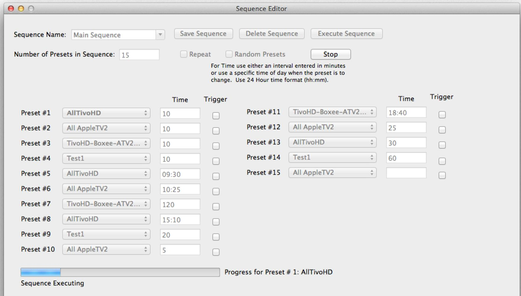
Sequences are time ordered sets of presets that change at a given time interval, time of day or a combination of both. They are available in the Pro and Custom versions of MediaSwitcher. Sequences can contain up to 20 presets. An unlimited number of sequences can be created.
