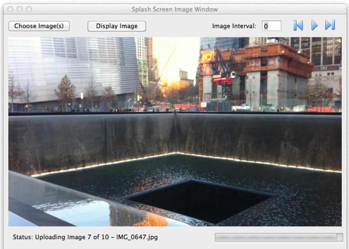
the image (at this time, all Just Add Power receivers display the images in 640x480 resolution). A progress bar showing upload progress along with the name of each images will be displayed on the bottom of the window.
