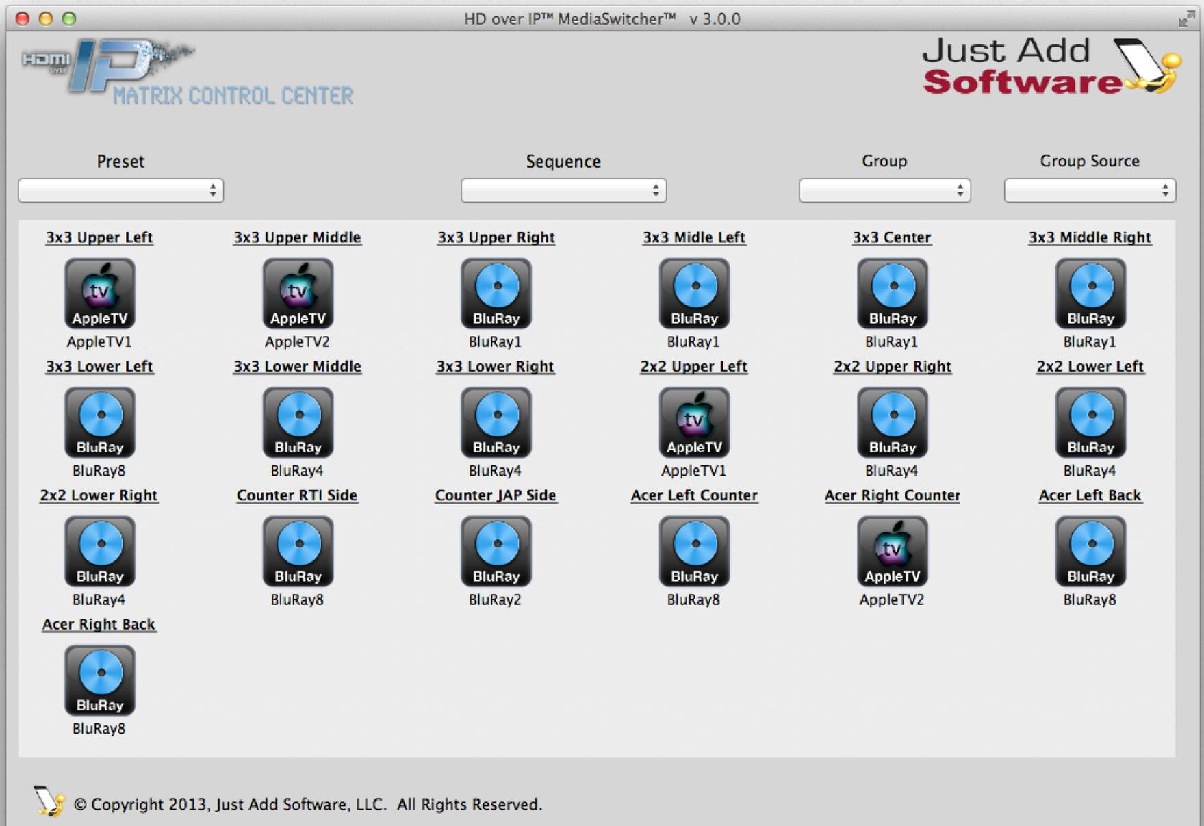
The main window is the center of all Media Switcher operations. From here, the video distribution is controlled as well as the ability to turn TVs on and off, control devices and more. The purpose of this chapter will be to associate the reader with the main features of this window and detail its operations.
