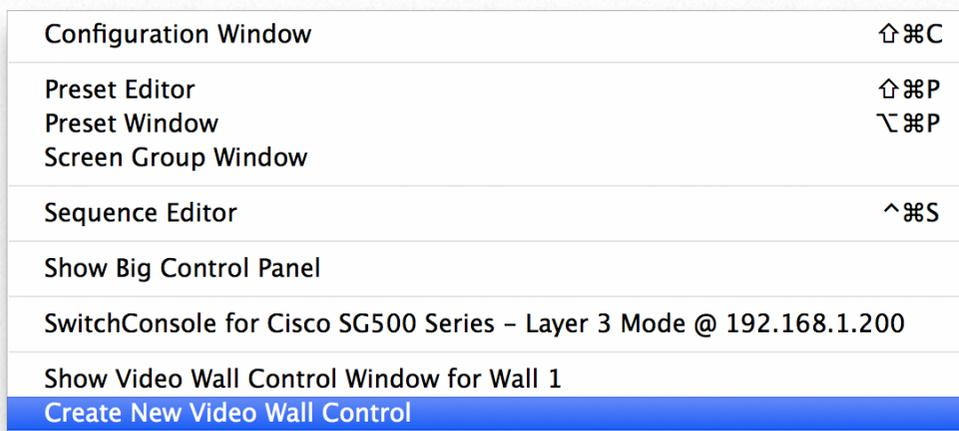
Once the control has been created, it will show in the menu and is numbered starting with 1. Additional controls for other screen matrices will be labeled, 2, 3, etc. Once a wall is created, it is not able to be deleted.
