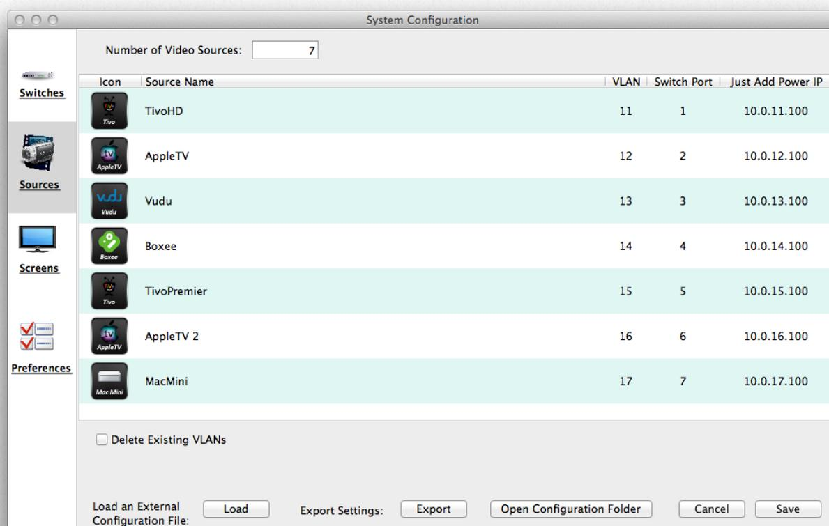
c.) Enter the port number on the switch that the transmitter is being plugged into.
