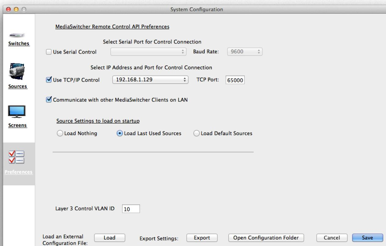
If RS-232 control is desired, select “Use Serial Control” and set the baud rate. Then connect the MediaSwitcher computer via RS-232 to your control system.
